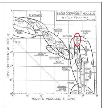
A classical benchmark for loudspeaker cone materials is the stiffness-to-weight ratio, which gives you the speed of sound in the material. Higher is better. See graph on the right side, magnesium is marked as a red dot:
